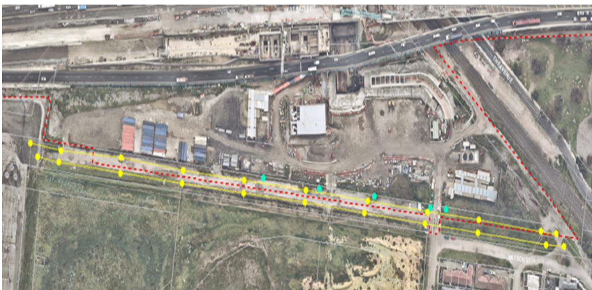
Figure 1: Plan showing 22 new HV poles (yellow dots) and wires in AusNet easement. Green dots indicate the existing poles.
