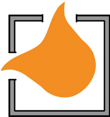
Two openings adjacent walls
