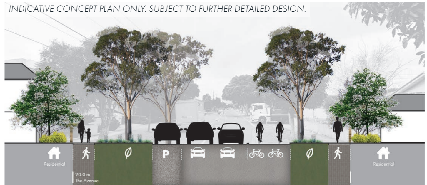
Figure 37. Proposed street cross section - The Avenue
