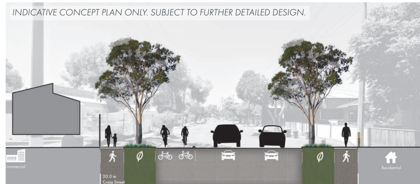
Figure 28. Proposed typical street cross section - Craig Street (between Hall Street and Douglas Parade)
