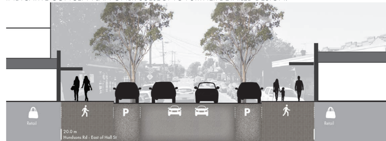
Figure 13. Proposed Typical Street Cross Section - Hudsons Road (between Hope Street and Robert Street)
