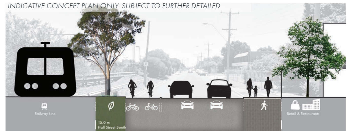
Figure 22. Proposed Hall Street Cross Section (section between Hudsons Road and Craig Street)
