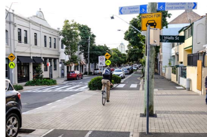
Example of a separated bike path improving safety at an intersection (above) and example of a different surface treatment used to delineate a shared intersection in a shopping precinct. (Source: City of Sydney)
