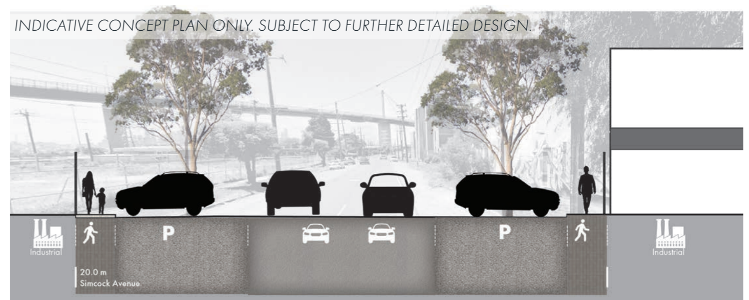
Figure 32. Simcock Avenue Typical Cross Section
