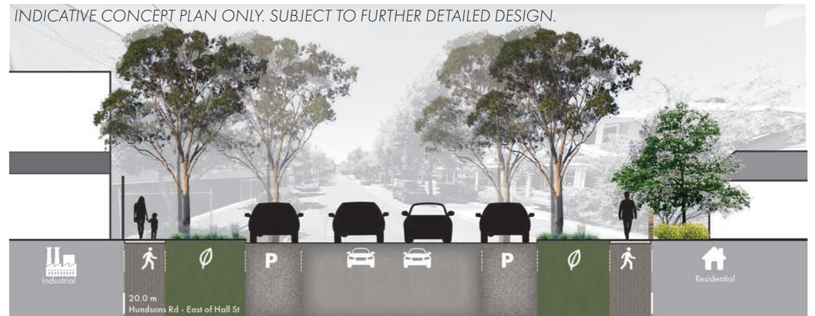
Figure 16. Proposed Typical Street Cross Section - Hudsons Road (between Hall Street and Booker Street)
