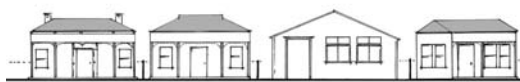
Figure 13. Bad example of infill, with inappropriate roof form and placement of openings.
