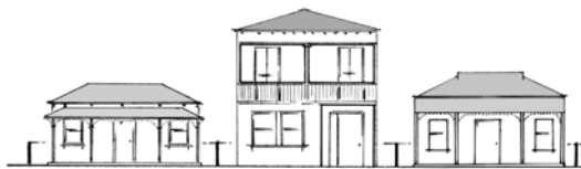
Figure 12. Bad example of infill, substantially larger than adjacent heritage buildings.
