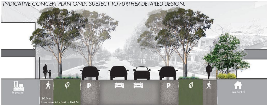
Figure 6: Proposed cross section for Hudsons Road East from Draft Spotswood Activity Centre Structure Plan, March 2022
