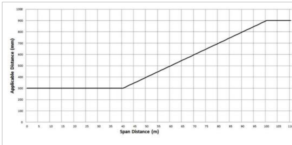
FIGURE 3—INSULATED ELECTRIC LINES IN ALL AREAS AND UNINSULATED HIGH VOLTAGE ELECTRIC LINES (OTHER THAN 66 000 VOLT ELECTRIC LINES) IN LOW BUSHFIRE RISK AREAS
