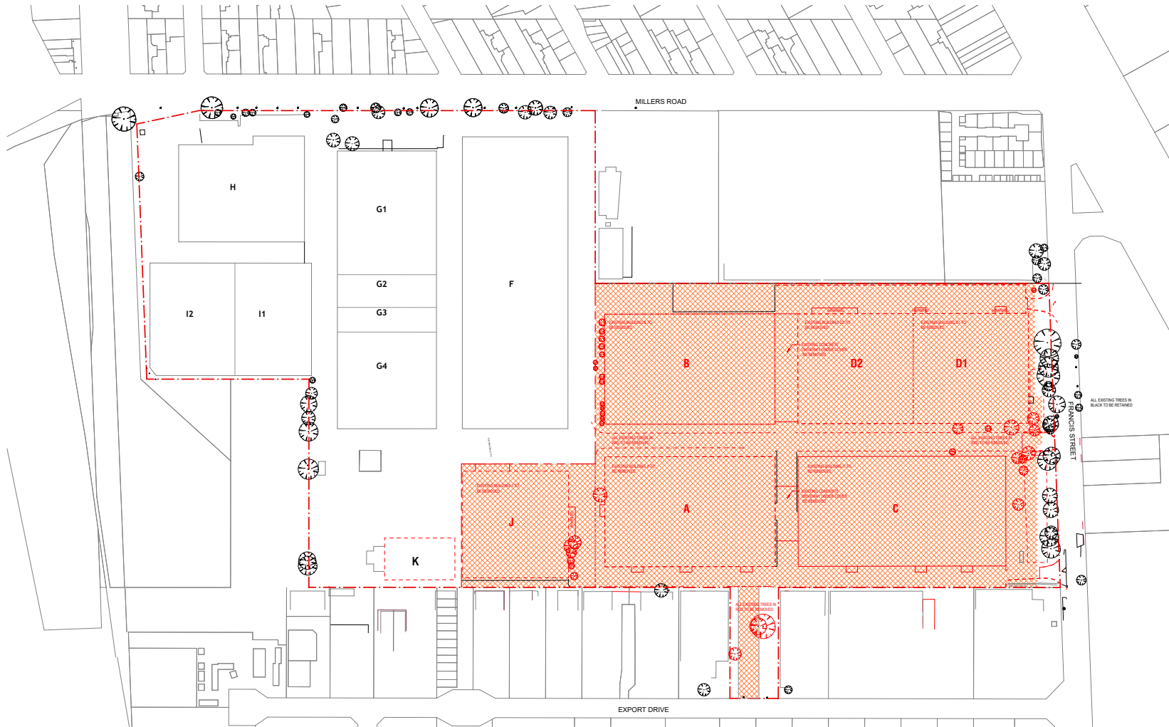
1 SITE PLAN - DEMOLITION 1:1000
