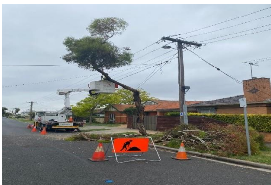
Image: New lift, allowing access to taller sections of trees for pruning works
