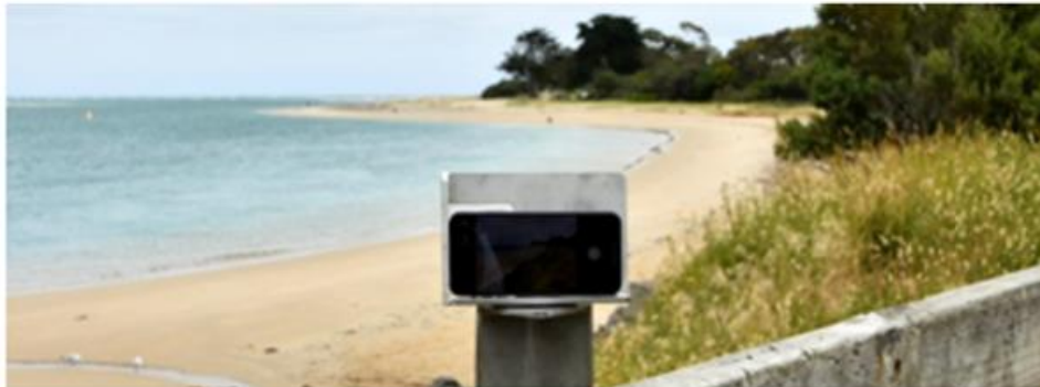
Figure 3: CoastSnap camera cradle
