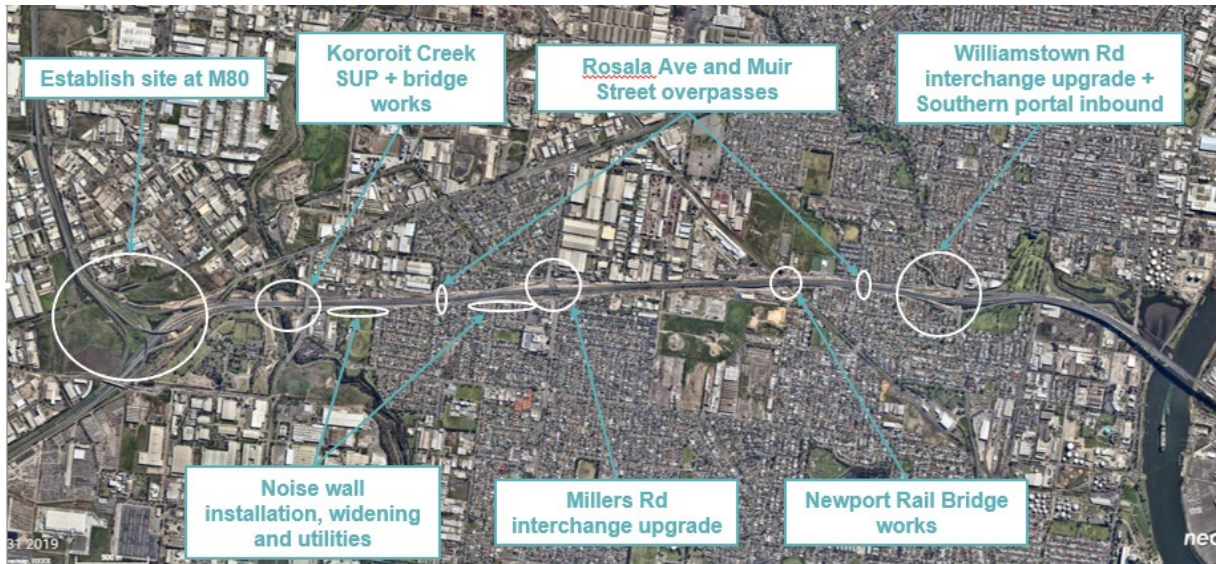
Figure 1: Current project construction activity
