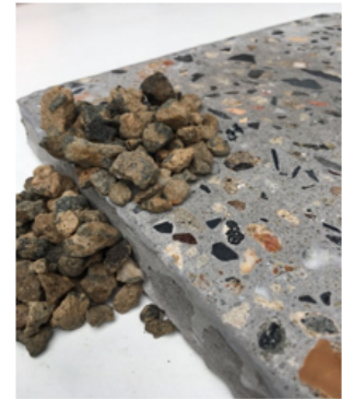
Recycled aggregates and concrete
